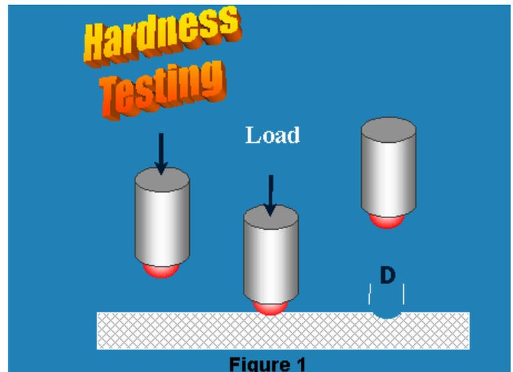
It's possible to think of this test as a **Macro Hardness** test. A **Micro Hardness** test on the other hand measures the individual hardness of each grain or particle.
