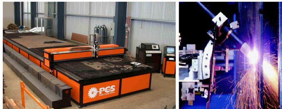
*Plasma-arc cutting is the recommended method of cutting overlaid plate*
