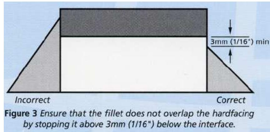
The easiest method for attaching Triten overlay plate to an existing structure is by a fillet weld. Care should be taken to ensure that the weld is applied to the substrate only and does not overlap the hardfacing or its penetration, as this can lead to carbon contamination and embrittlement of the weld. This is best achieved by stopping the fillet approximately 3mm (1/8") below the alloy/base plate interface which should be clearly visible on a ground edge. See figure 3.
