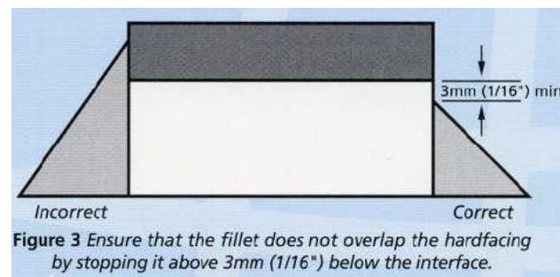
**Figure 3** Ensure that the fillet does not overlap the hardfacing by stopping it above 3mm (1/16") below the interface.
