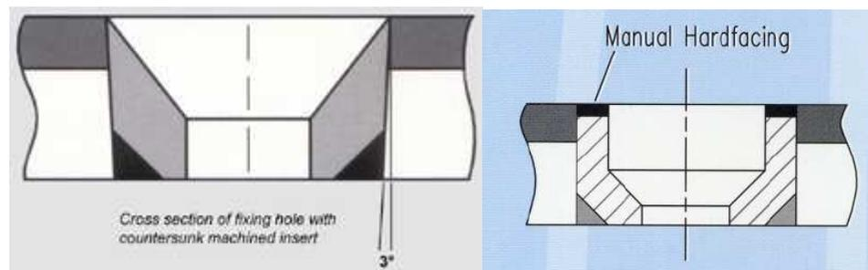
**Gouging** - this process is generally used on-site when plasma-arc cutting is not available. If a large number of holes is required, welded inserts are recommended and gouging should be used purely to cut the clearance hole.
