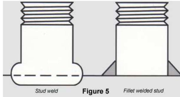
A standard carbon steel stud can be easily welded to the back of the Triten overlay plate using most types of stud welding equipment. The minimum recommended stud size is 19mm (3/4") and the number and spacing of the studs will depend on the size and shape of the plate being attached.
