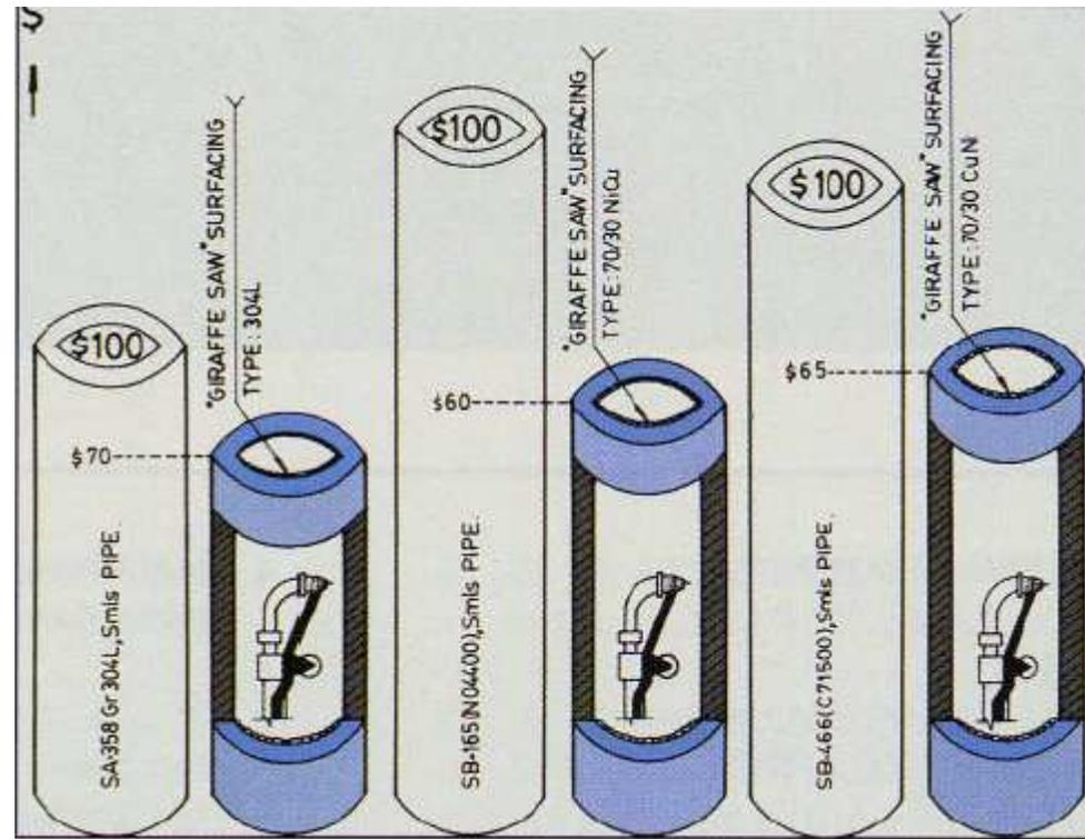
Fig. 1. Cost comparison chart of solid pipe versus SAW internal weld surfacing.
