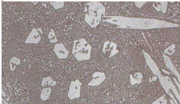
200x magnification Average Hardness HRC 51,87
